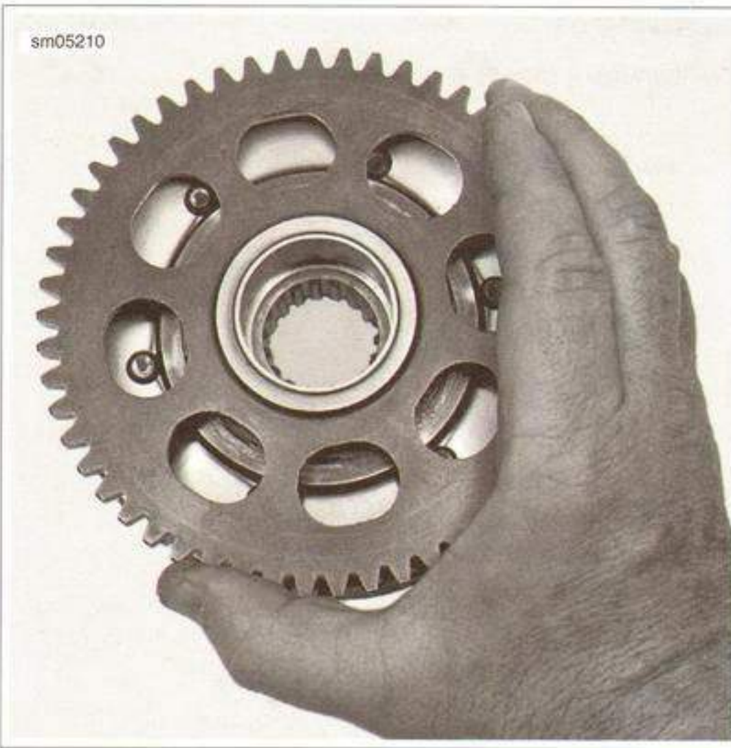
Figure 7-37. Rotate Starter Gear to Fit Sprag Clutch
