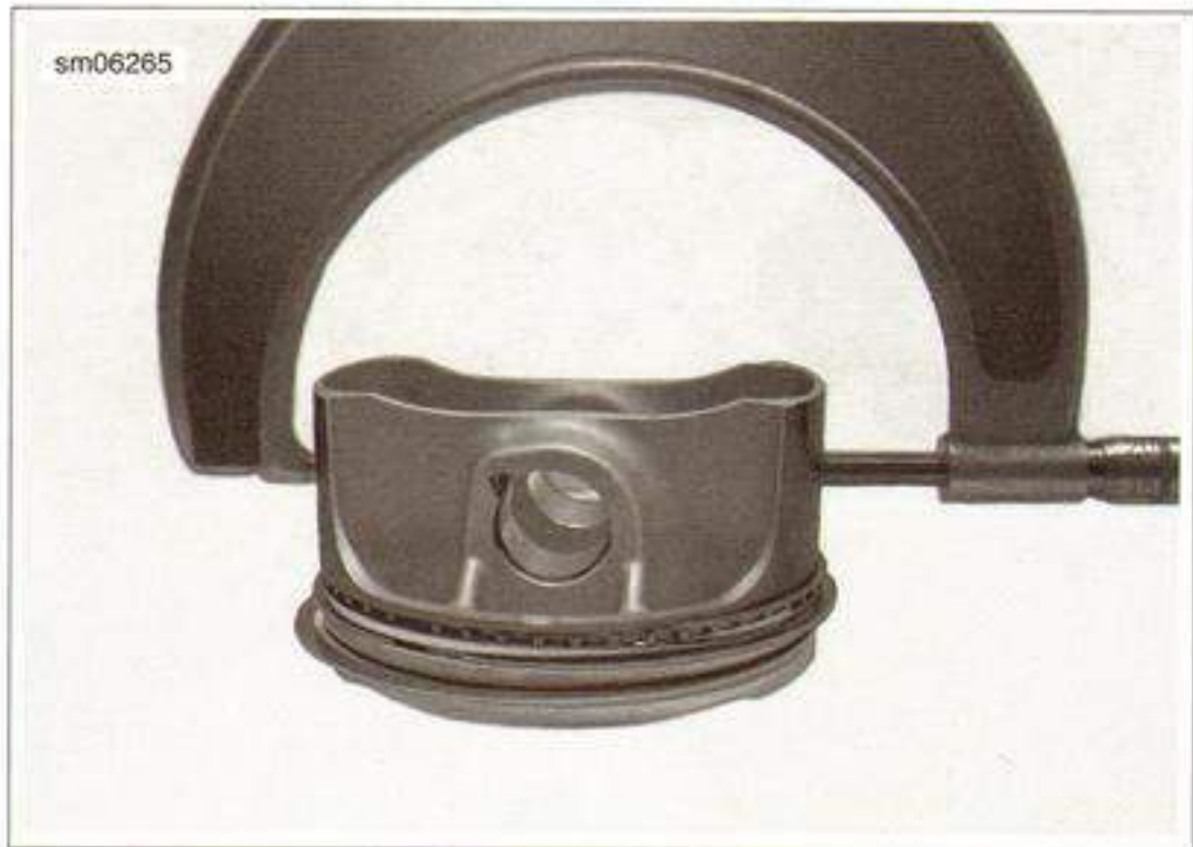
Figure 3-100. Measuring Piston Diameter
