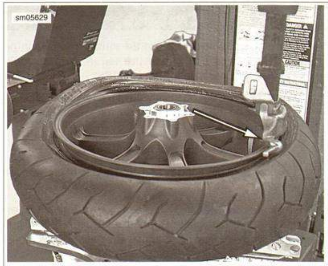
Figure 2-16. Feeding the Upper Bead onto the Rim
