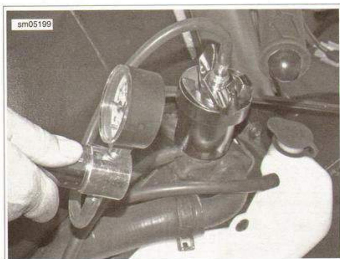
Figure 5-5. System Pressure Test
