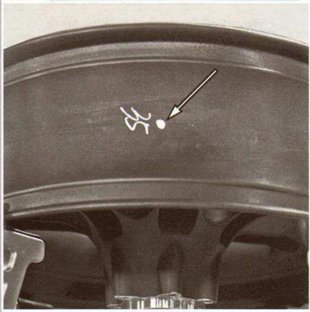
Figure 2-15. Tire and Wheel Balance Dots
