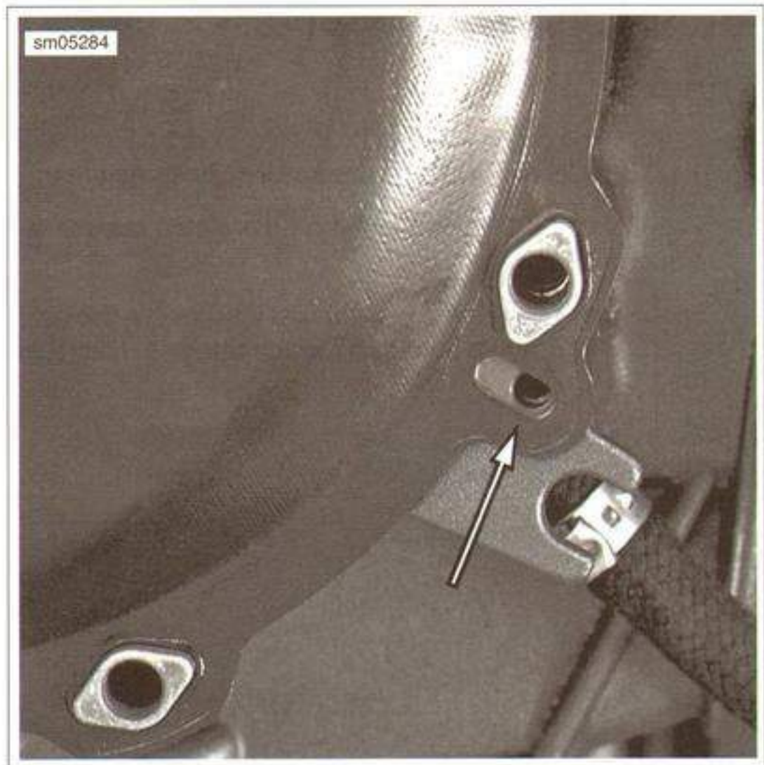
Figure 6-33. Gasket, Inner Cover and Diaphragm Alignment
