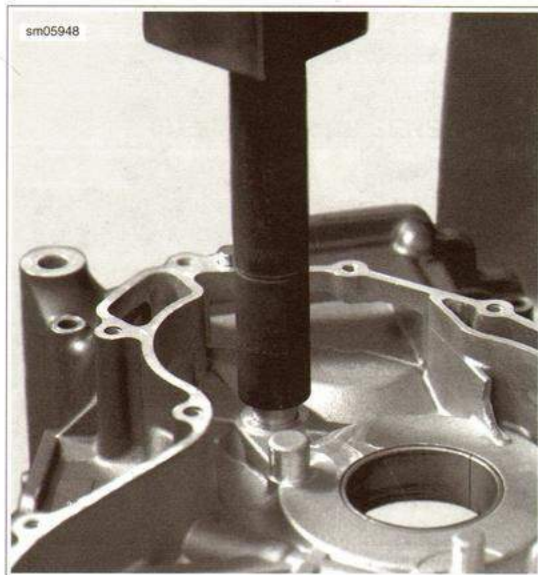
Figure 3-182. Water Pump Shaft Case Bearing Installer (B-49403)
