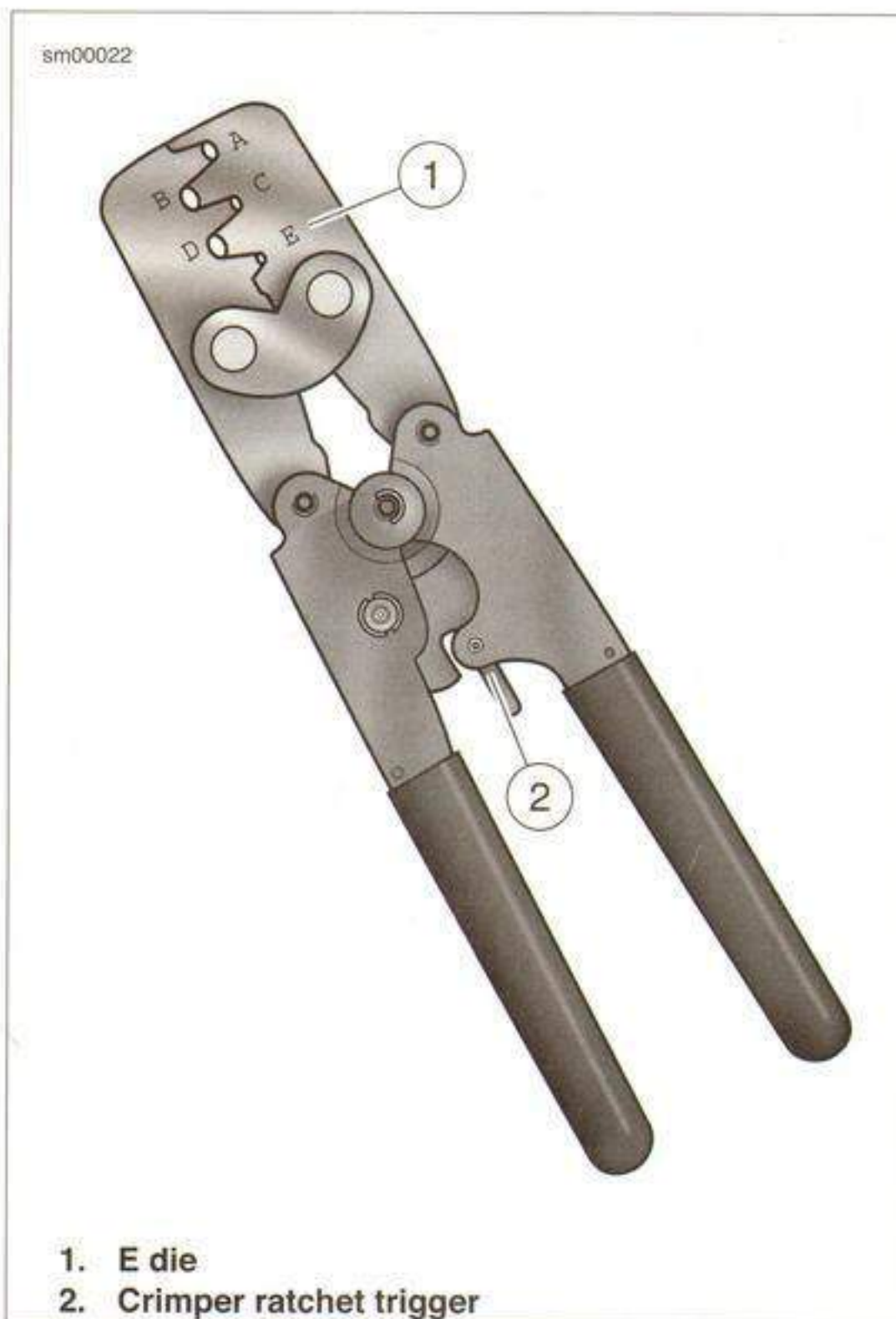
Figure A-24. Packard Terminal Crimper (HD-38125-7)
