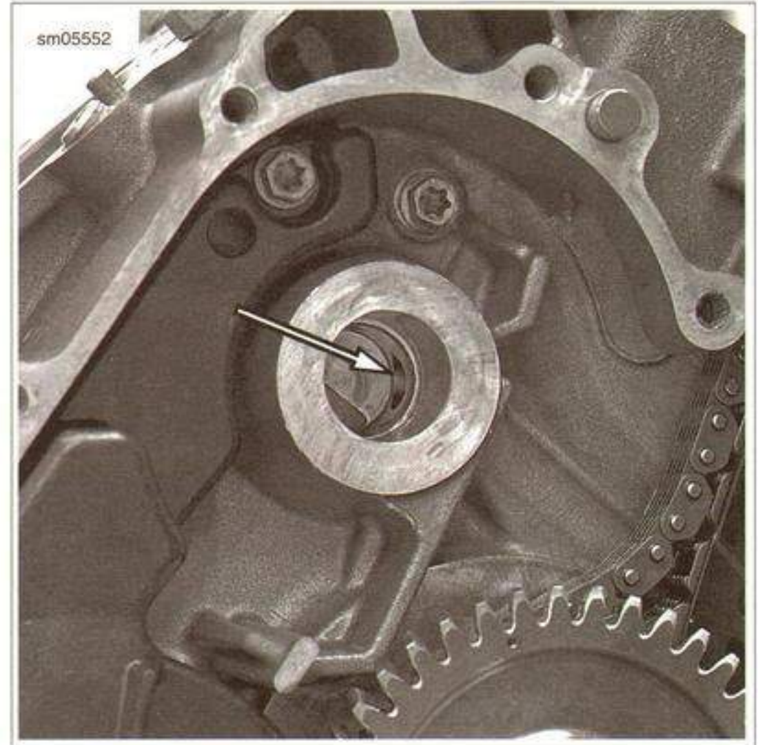
Figure 3-150. Oil Passage in Balancer Support in Crankcase
