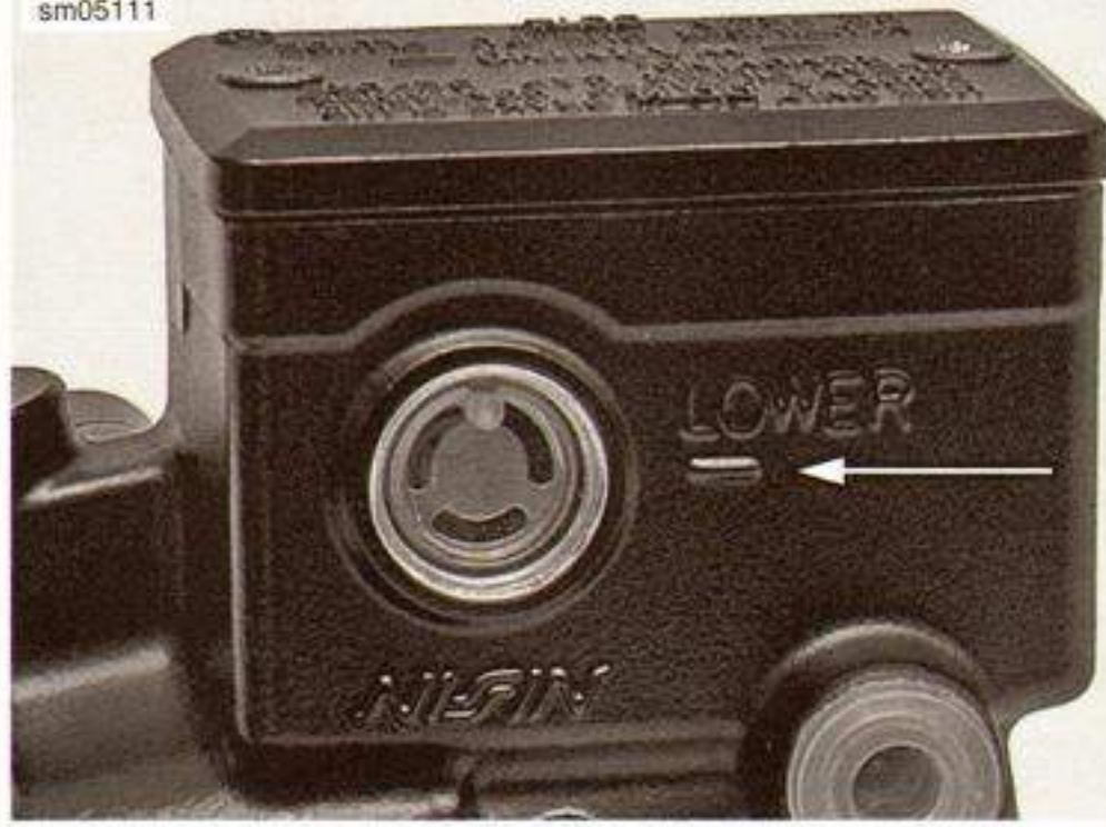
Figure 1-19. Brake Fluid Reservoir LOWER Line
