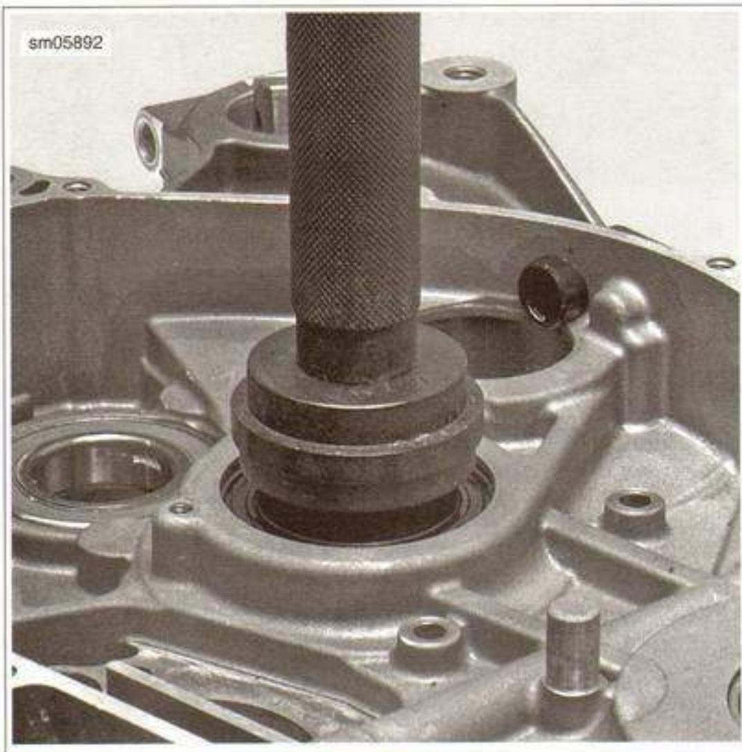
Figure 6-101. Clutch Shaft Bearing Removal: Right Case
