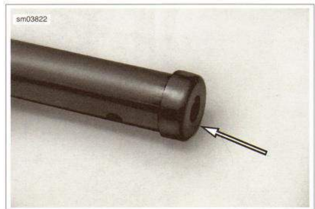
Figure 2-92. Centering Plate on Bottom of Damper Rod
