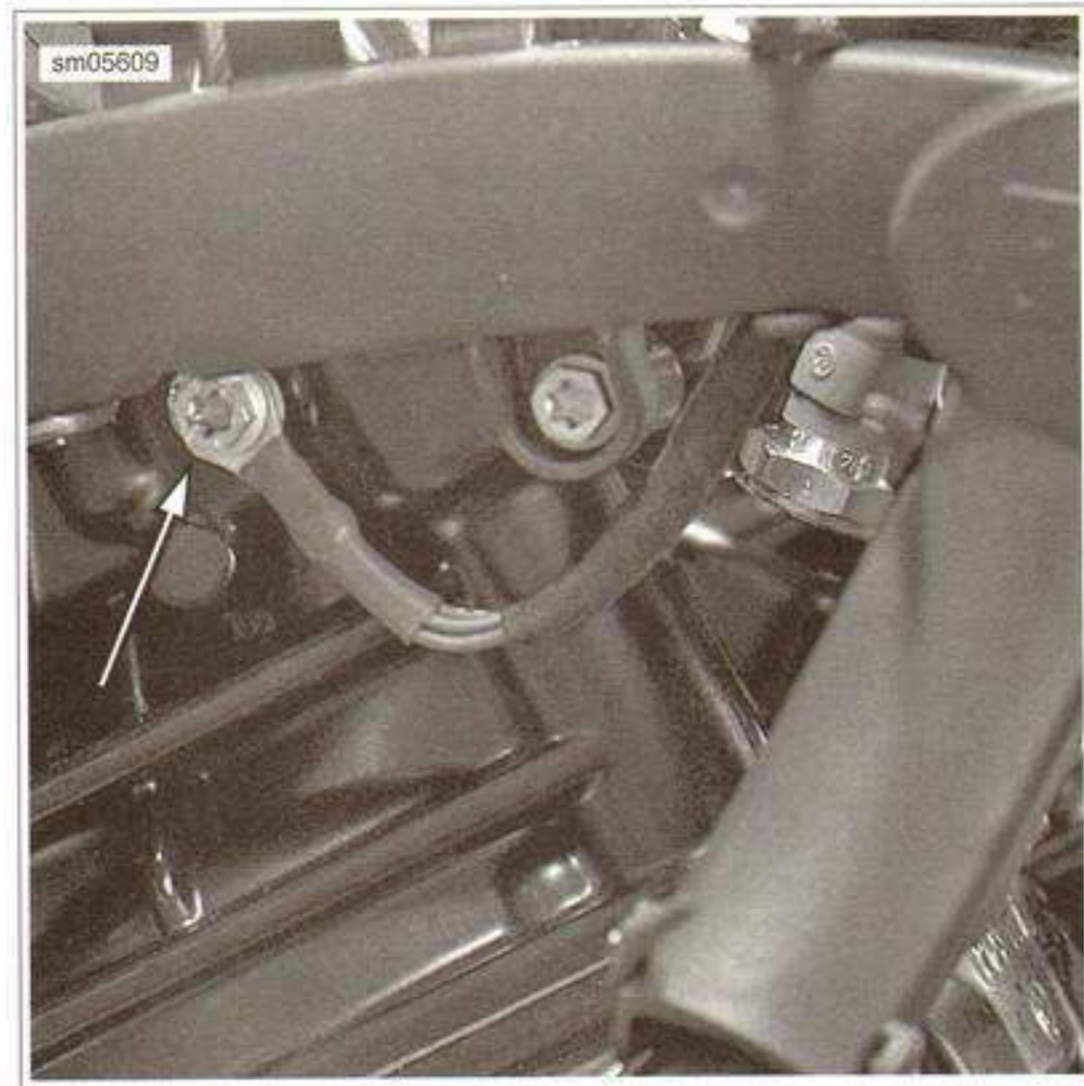
Figure 7-108. Engine Ground Connection
