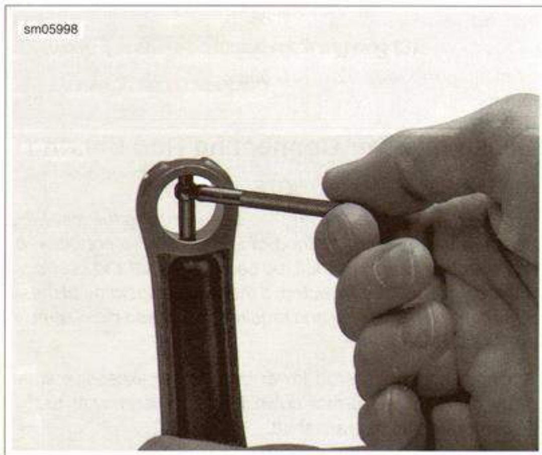
Figure 3-97. Connecting Rod Piston Pin Bore Measurement
