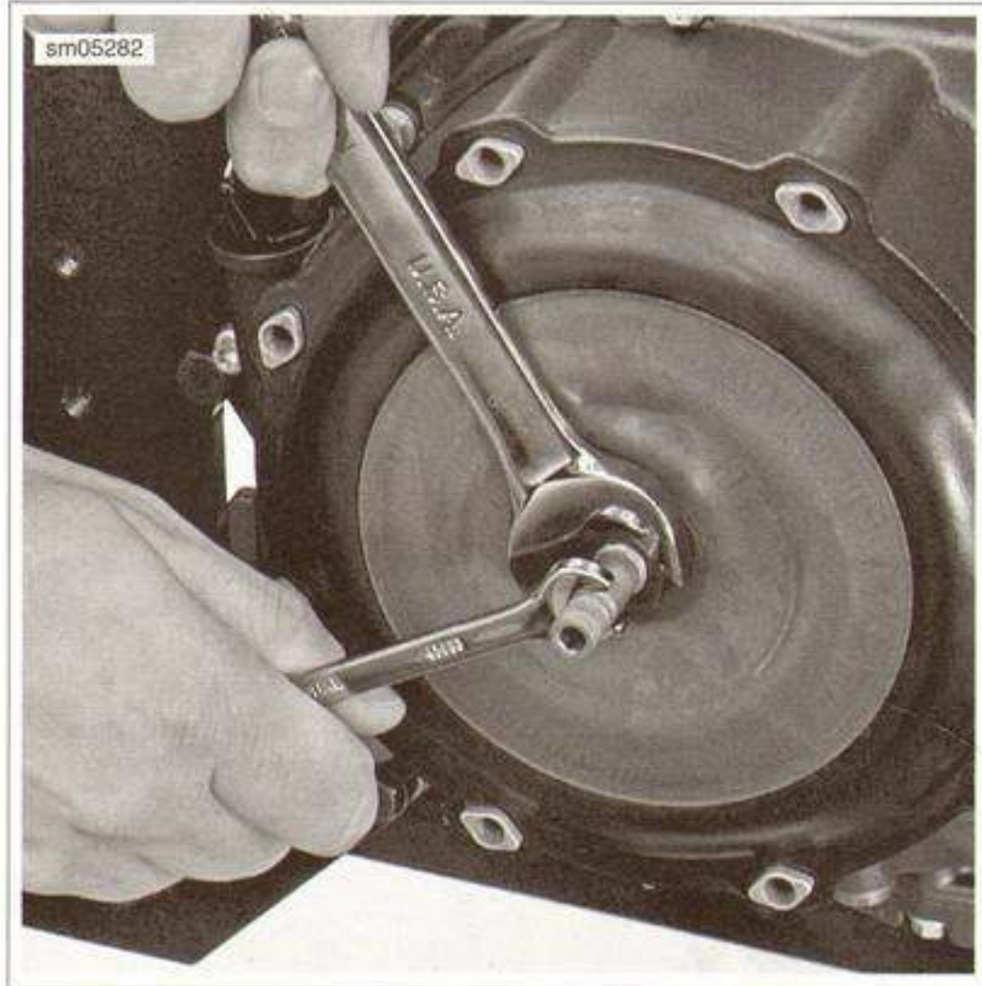
Figure 6-29. Removing the Neck Nut from the Clutch Release Pin
