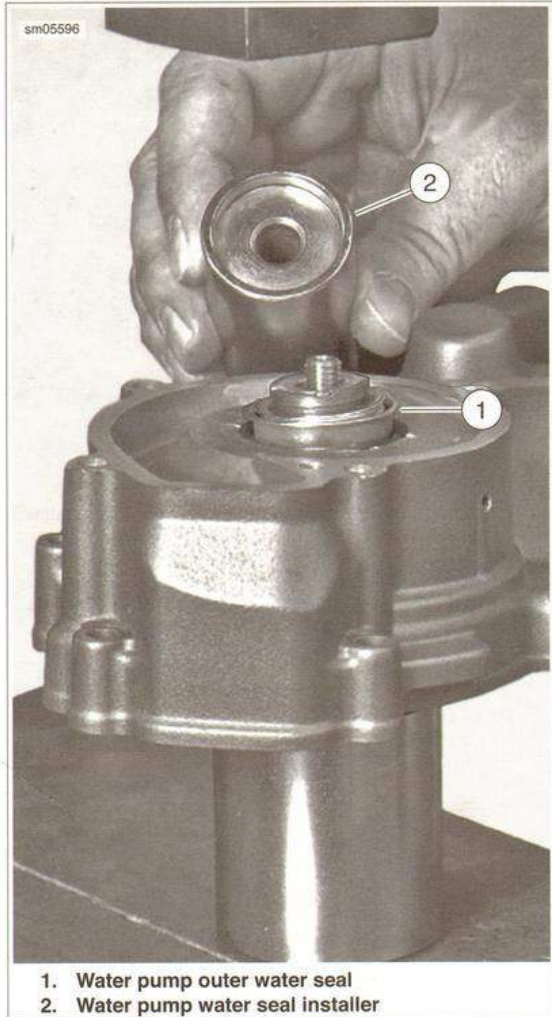
Figure 5-21. Position of Outer Water Seal and Installer Shoulder
