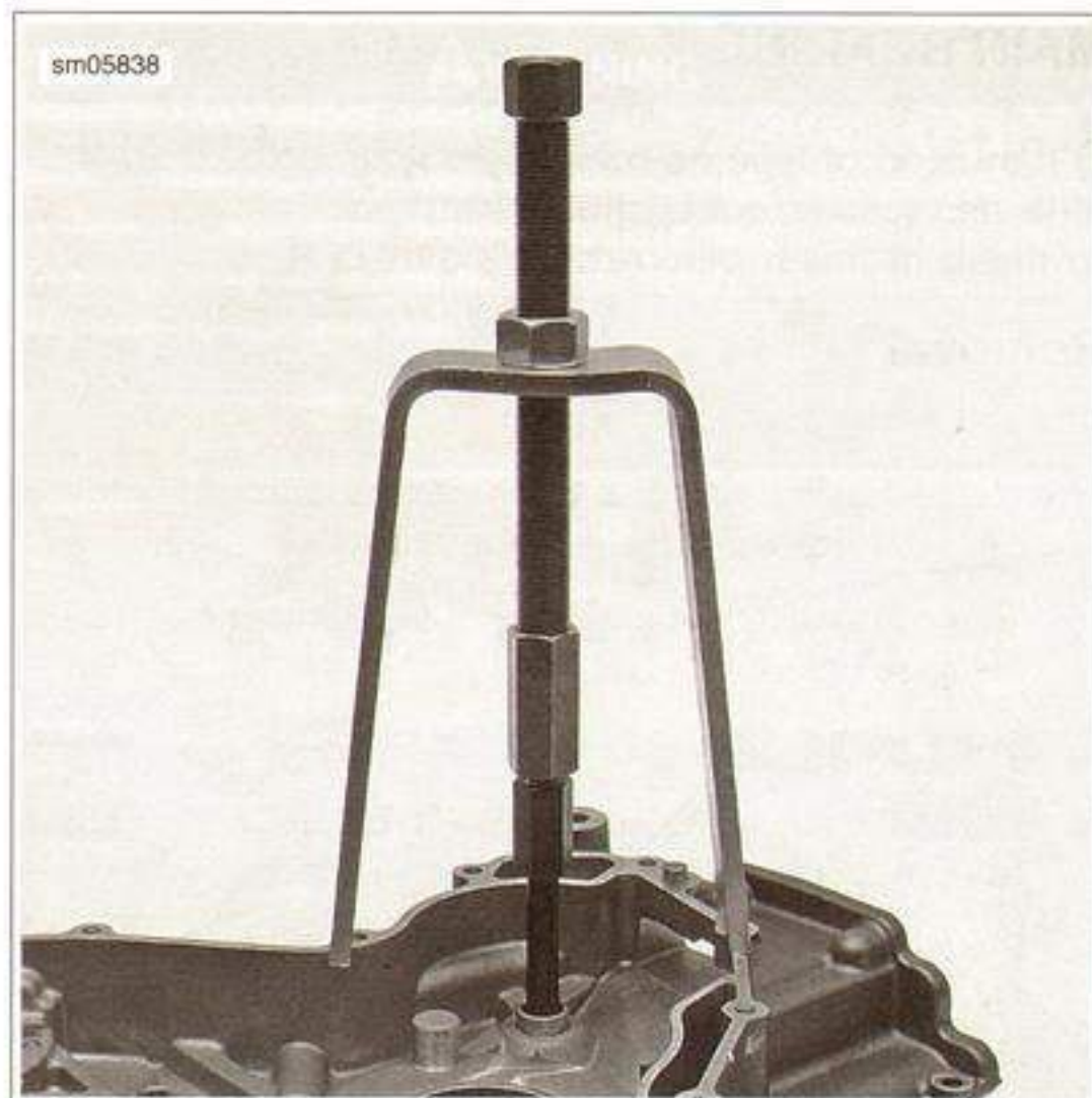
Figure 3-181. Remove the Water Pump Shaft Case Bearing
