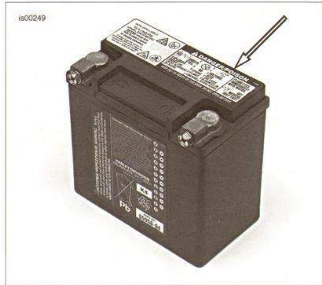
Figure 1-46. AGM Battery with Warning Label
