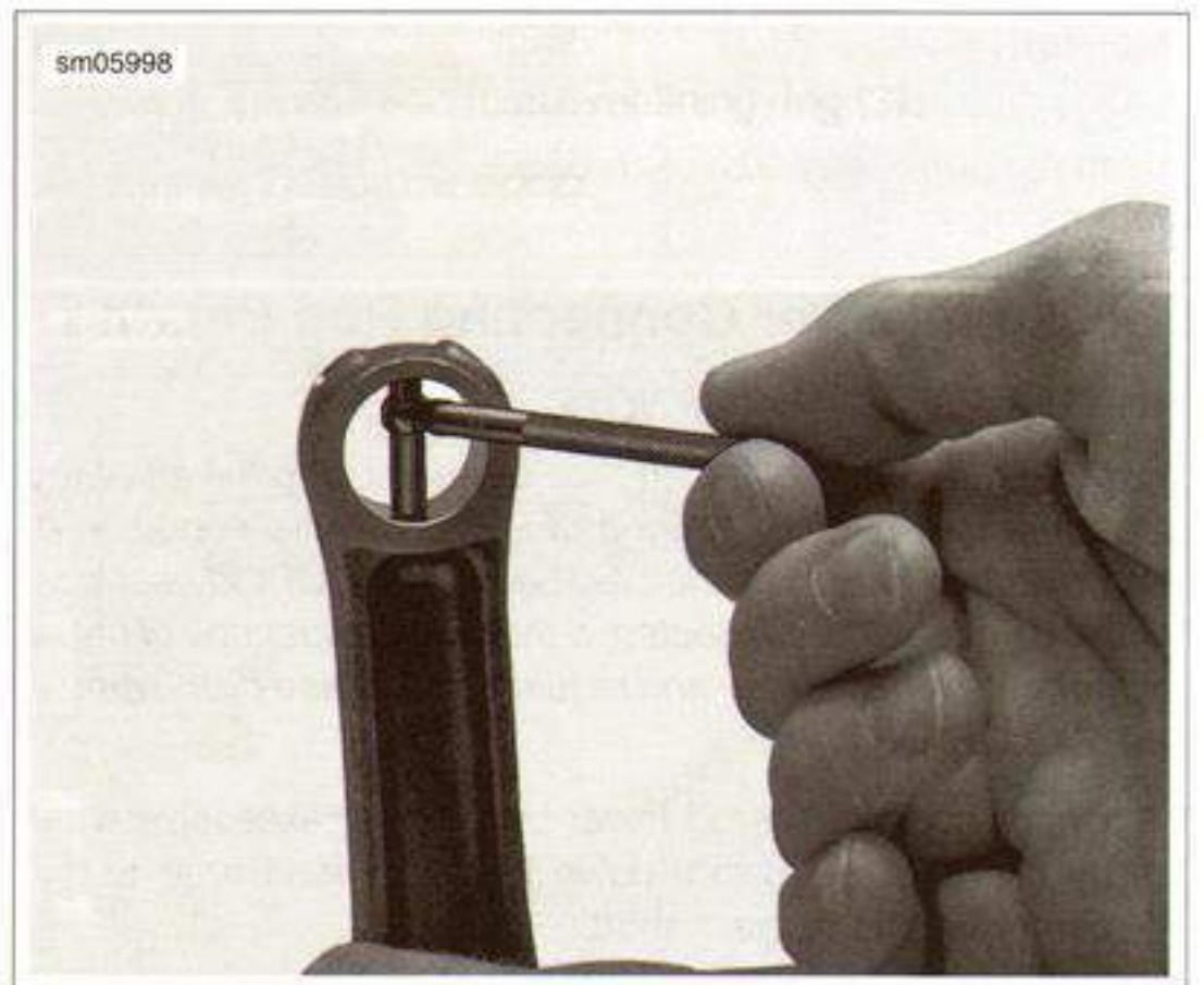
Figure 3-97. Connecting Rod Piston Pin Bore Measurement
