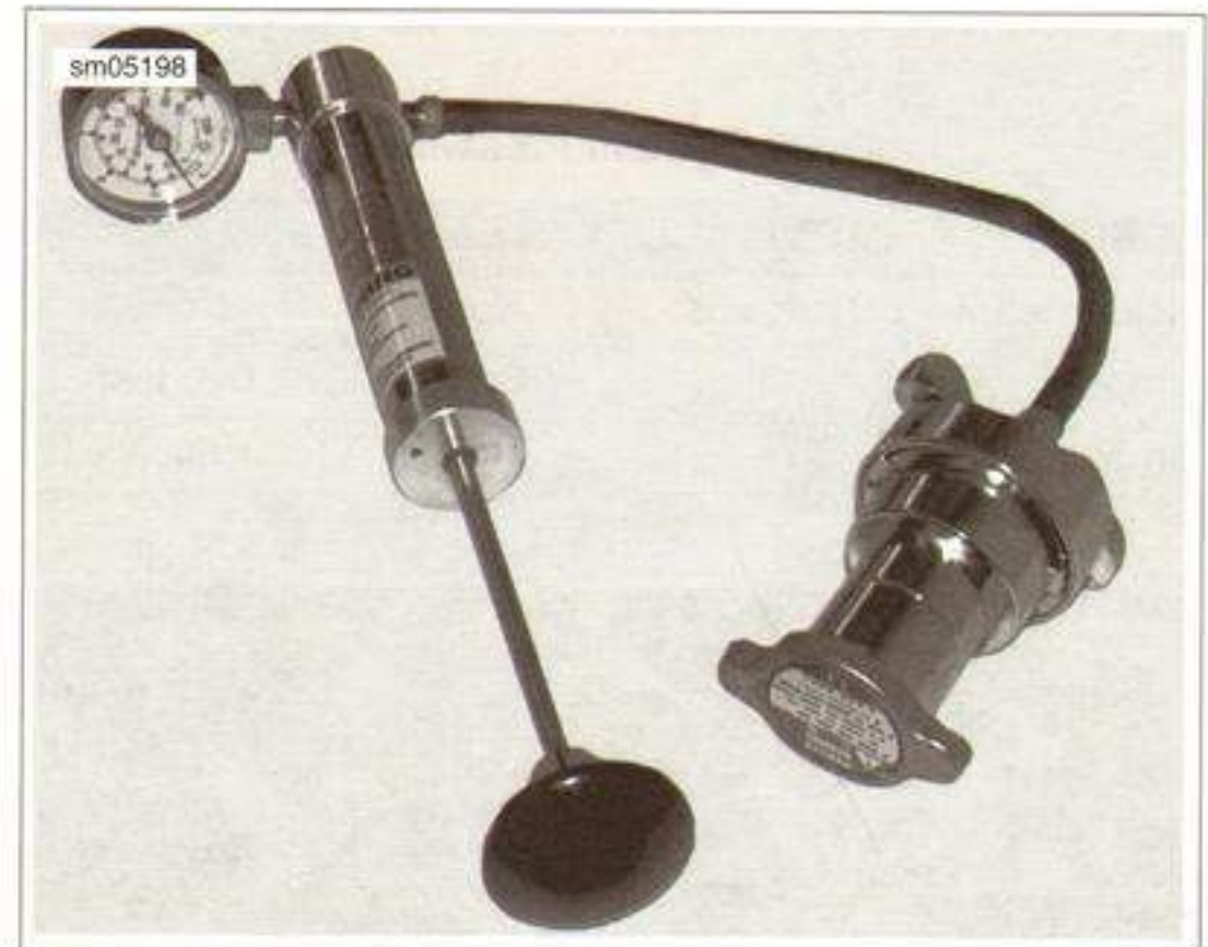
Figure 5-4. Pressure Cap Test
