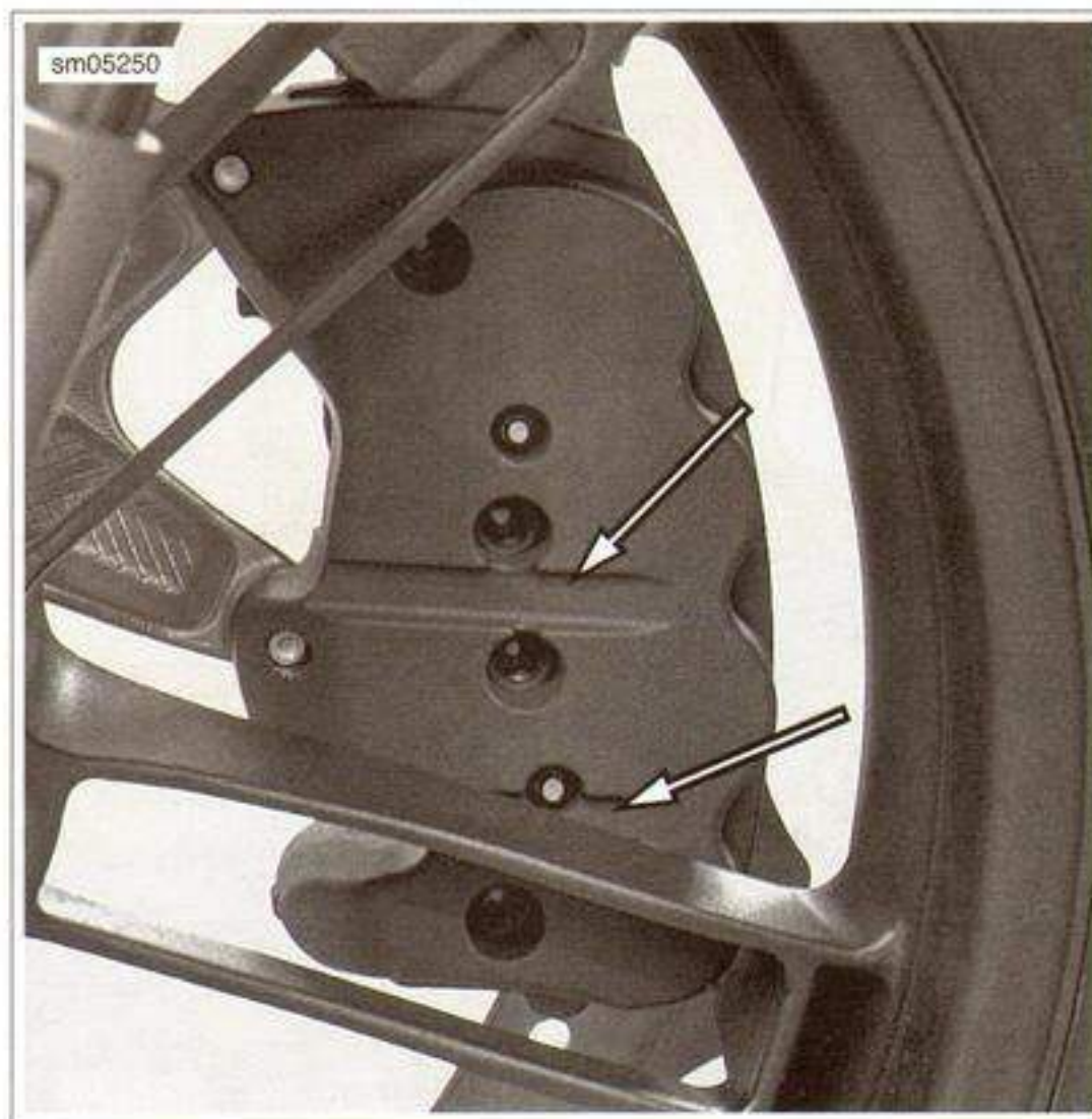
Figure 2-20. Caliper to Spoke Clearance Slots
