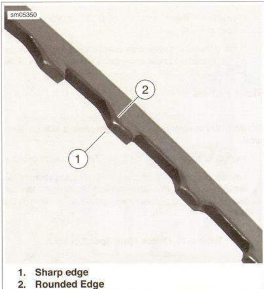
Figure 6-43. Sharp and Rounded Edge Steel Plate
