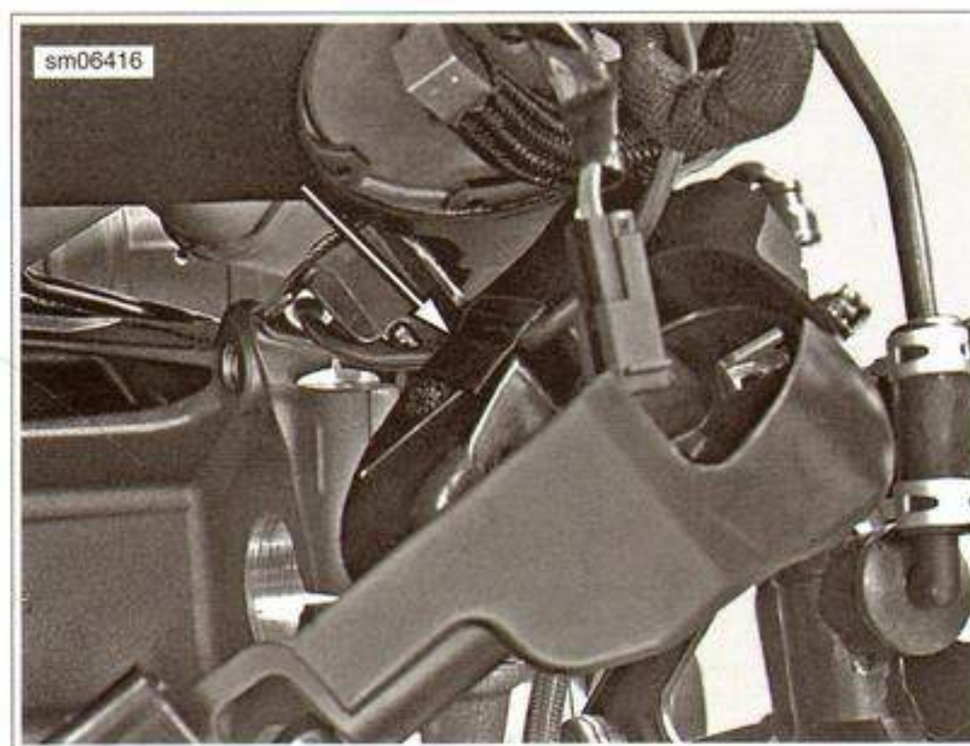
Figure 4-68. VSS Lead Taped in Cover
